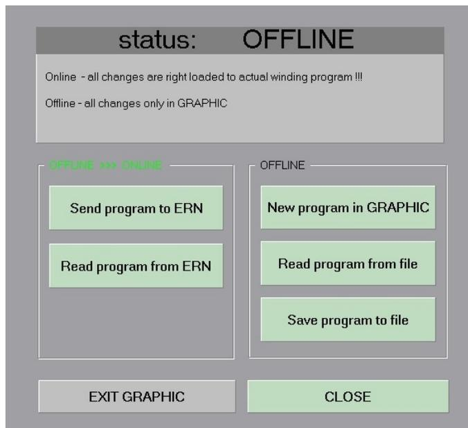
**Send program to ERN** - Winding program which is opened in the memory of the Graphic, we send it in to the winding machine ERN, thus with this action we rewrite actual running program and at the same time the mode is switched to ONLINE. Here we can run this program or correct it straight in the winding machine.
