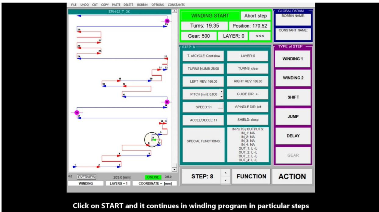
*Note:* for models that allow to programmatically switch GEAR (e.g. ERN 62), we recommend programming in step no. 1 switching the initial gear and in step no. 2 program shift to the coordinate where we start winding
