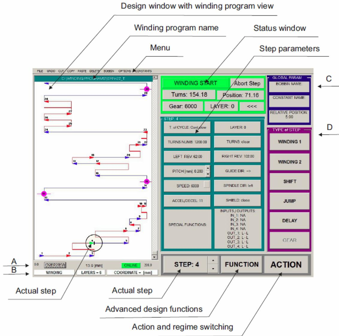
A: Left coordinate of design window (mm), Mode of view, actual maus position (mm), Work mode, Right coordinate of design window (mm)
