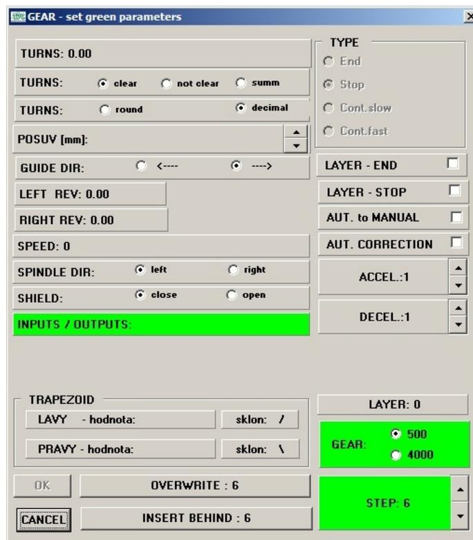
To be able to automatically switch the gears, this possibility must be allowed in switch gear settings, which are displayed on the screen right after winding machine is turned on. It is necessary to set GEAR FROM PROGRAM. After this option is activated and after the winding machine is turned on, it will change the gear to lower RPM and continue to manage the gear set by the winding program.
