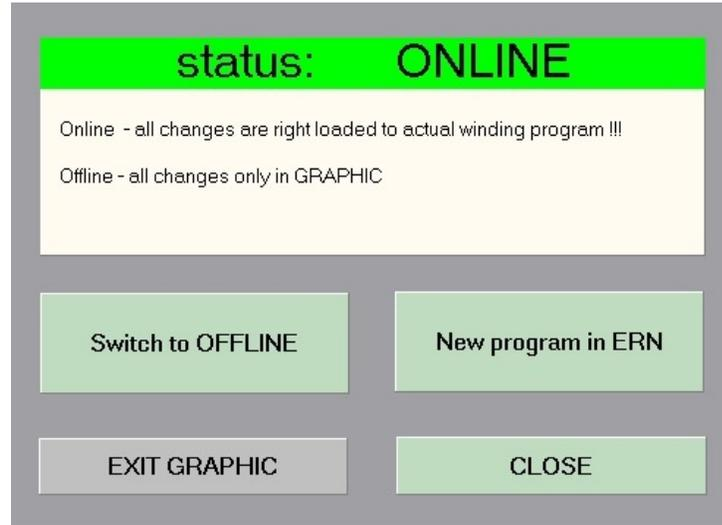
**New program in ERN** - Erases currently running program in the winding machine and we can write the new one.
