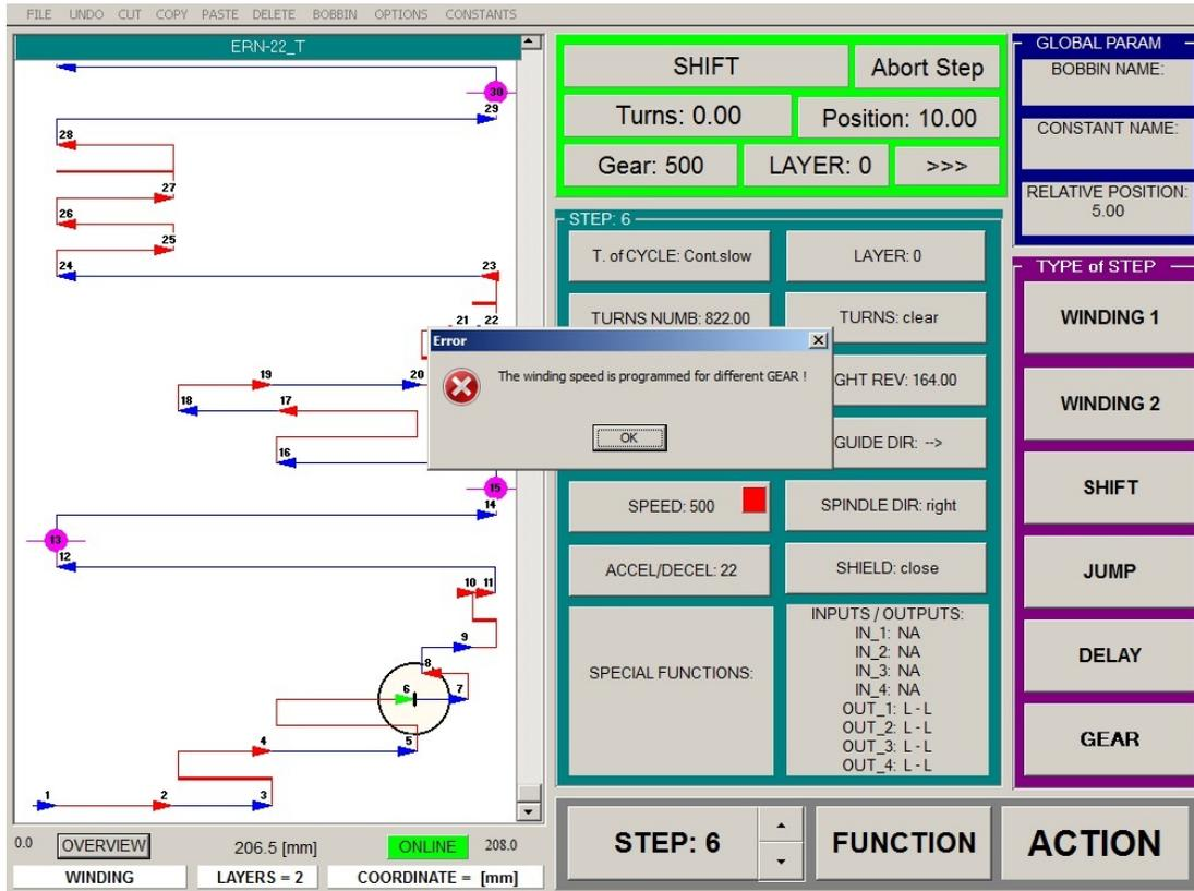
Note: If the winding program with the option of automatic switching of the gears is copied to model of winding machine without the option of automatic switching of the gears, then the winding step GEAR is ignored. Newer models of machines will show error message FIXED GEAR SET.
