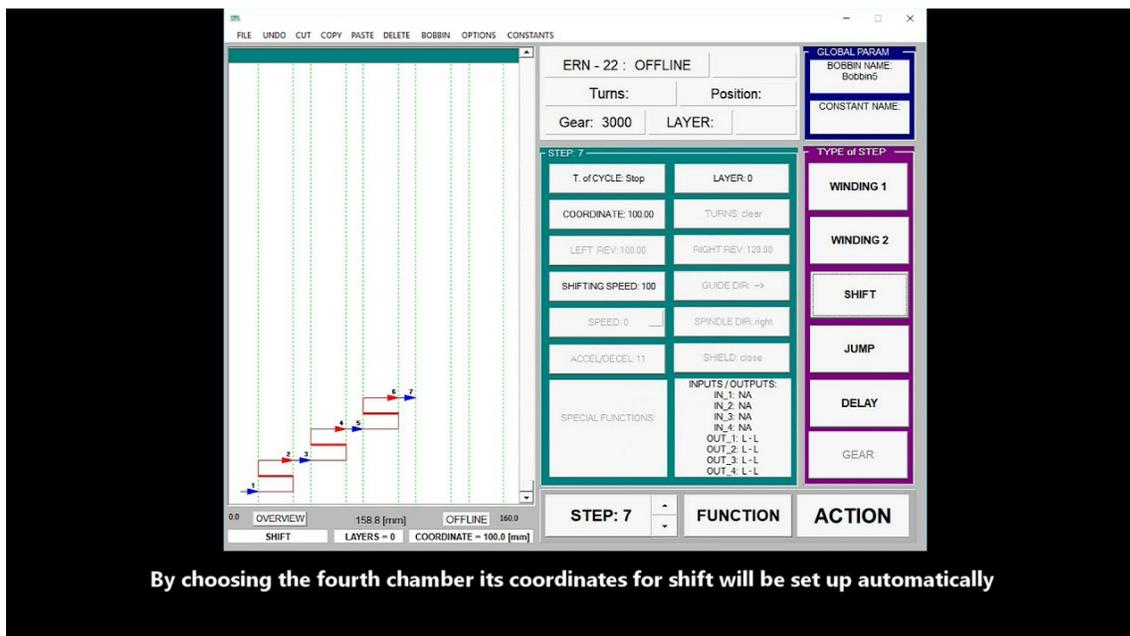
By choosing the fourth chamber its coordinates for shift will be set up automatically
