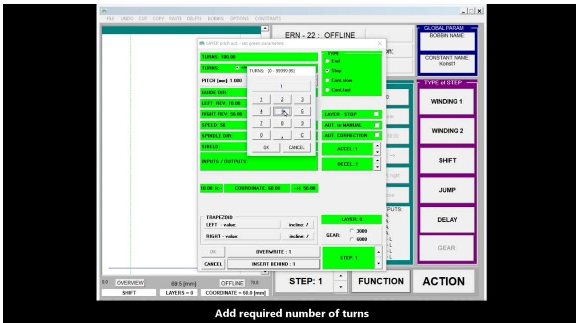
At the specified number of turns, the function calculates the required pitch so that we get to one of the reversal points, which we determine by setting the direction of the guide. The function can overwrite the current step or insert a new step.
