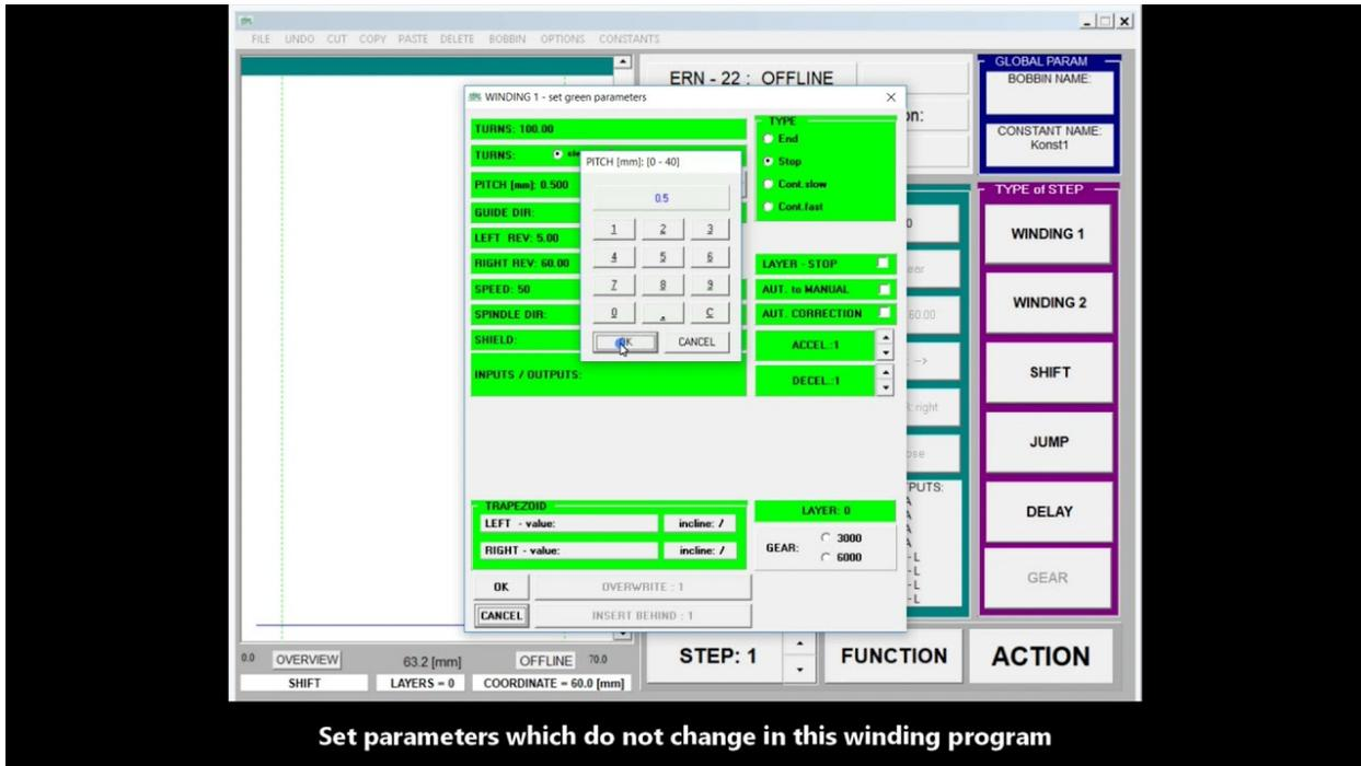
3. We will start programming individual steps of winding program, and we strongly recommend that the first step of program be shift to the coordinate where we start winding.
