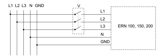
An additional switch "V" is recommended to use in case, if the lead-in cable is fixly connected to the line distribution. If the moving terminal is used for the installation, this switch will be not necessary.
