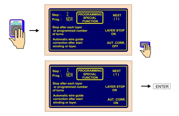
After the first layer is wound (e.g. from left to the right), press the wire guide correction button and correct the wire guide position. This corrected position is saved by pressing SAVE AS RIGHT CORRECTION button. Likewise, we insert and save the left correction after the second layer (from right to the left) is wound. For all the following layers in this step, all the corrections are done automatically, after start.
