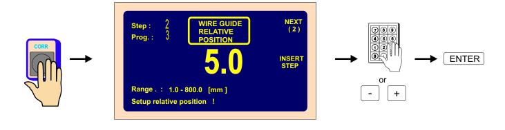
Holding the buttons - + pressed (cca 0,5 s) moves the wire guide continuously.
