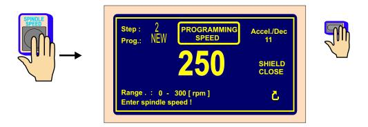
Entry of values 1 to 8 for acceleration and deceleration according to the enclosed table.
