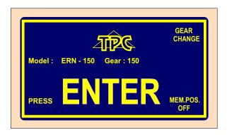
which provides informations about, for what type of machine is controller set. In this window we can change the set gear, which must be in ABSOLUTE ACCORDANCE with the set of mechanical gear.
