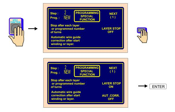
Until programmed number of turns is not reached, machine stops after each layer on the left or right reversal point.
