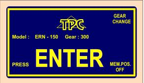
After pressing ENTER-button, the initial set is done, which means, that wire guide is shifted left home (zero position), zero number of turns, zero step and the last program is set.
