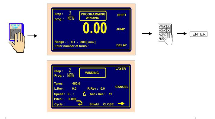
If " 0 " is programmed to the number of turns, this winding step turns the spindle to the zero reference position. Direction of the spindle speed is taken from the previous winding step!
