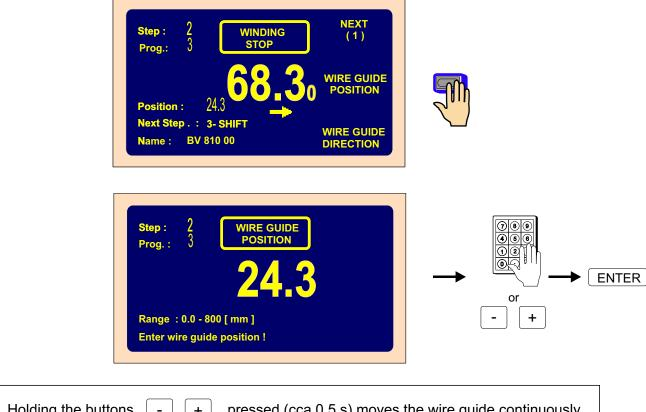
Holding the buttons - + pressed (cca 0,5 s) moves the wire guide continuously.
