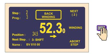
Pressing of multifunction button "WINDING" ends back winding.
