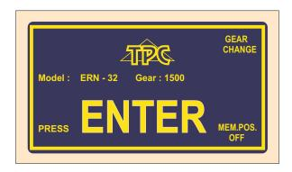
which provides informations about, for what type of machine is controller set. In this window we can change the set gear, which must be in ABSOLUTE ACCORDANCE with the set of mechanical gear.
