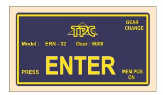
After the activation of this function (MEM.POS.ON) the initial setting will be actualized for the values, memorized while electricity drop.
