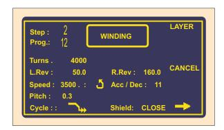
Winding is possible only in these two windows. If any other window is opened, the cycle start is blocked.
