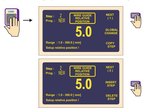
Position for step insertion is chosen by buttons
