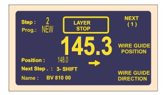
Maximal value for wire guide correction can not overreach  $\pm$  10 mm position diversion, after the layer is wound. Higher values are not accepted!
