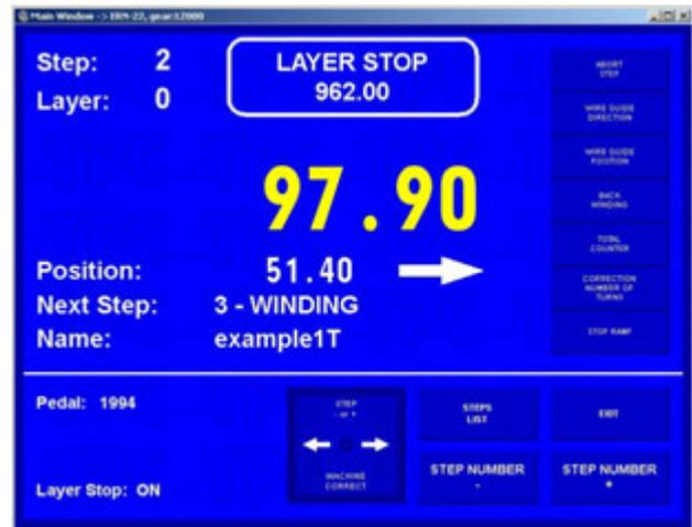
Maximum value for wire guide correction can not be greater than  $\pm 10$  mm after a layer is wound. Value higher than this will be ignored !
