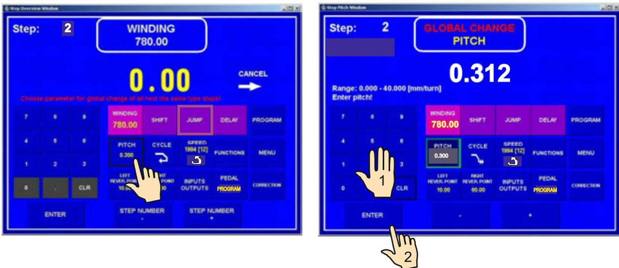
The pitch is changed in all the subsequent winding steps.
