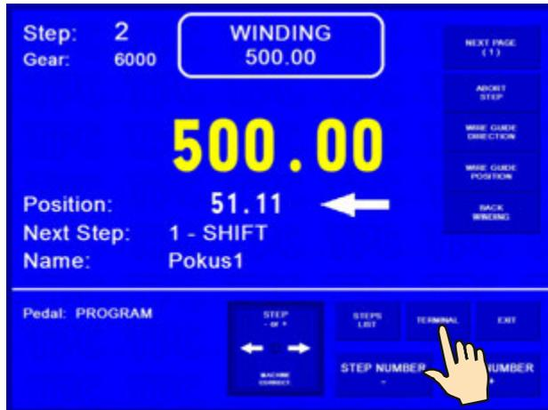
Winding procedures are able to provide winding machine operators with additional important information on winding. If a winding programme is accompanied with a corresponding winding procedure a current winding step technological operation description is displayed on the winding machine monitor automatically. This information comes from the winding procedure and it can be represented in form of texts or images.
