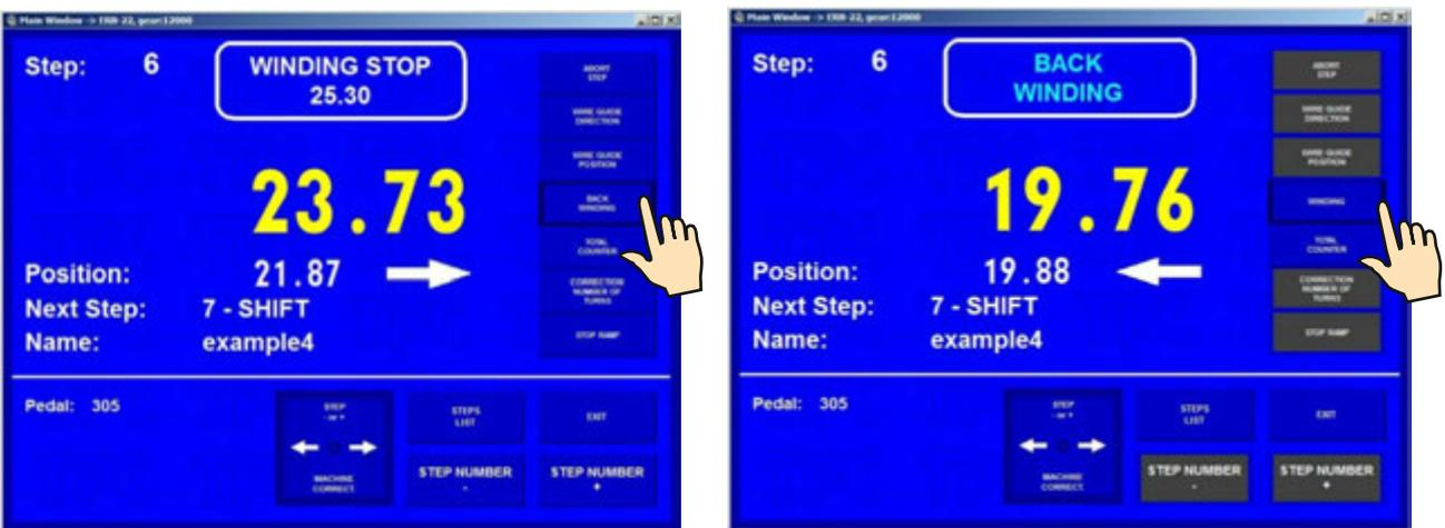
We can wind back the number of turns required only by using the pedal. The number of turns is counted back and the wire guide moves in opposite direction.
