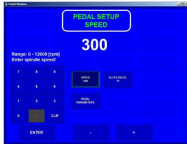
Speed set up in this way is applicable only for the current programme. It is independent of the speed programmed in a specific programme step. Eg.: maximum speed set up by START pedal may be differ to maximum speed set up by START button.
